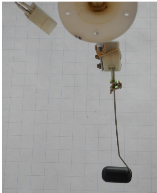
Figure 9: Float in normal position
