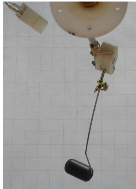
Figure 10: Float in skewed position
