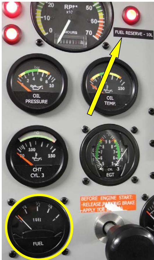
Figure 1: Fuel gauge (yellow circle) and red FUEL RESERVE warning lamp (yellow arrow)
