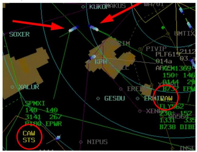
2. In EPWA APP system the STCA settings were identical to the ACC system where the lateral separation is 7 NM (for APP 3NM/5 NM). This meant that the situation which was absolutely correct repeatedly activated the alarm.
