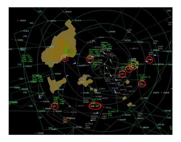
Each of these warnings was visualized in a color attracting attention (yellow or red, and SPi – white flashing) which means that at the same time they diverted the Controller's attention from other elements shown on the screen.
