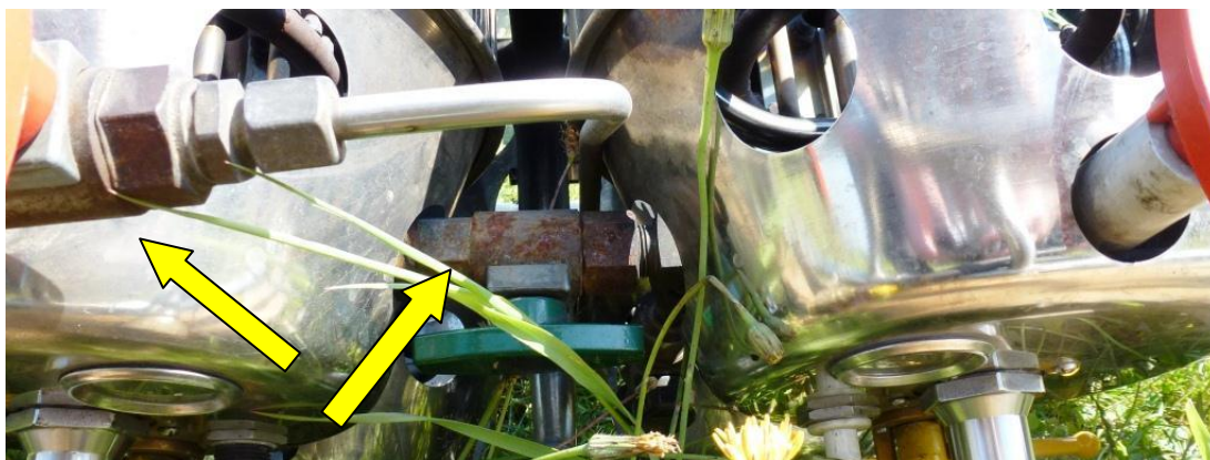
Photo 3. Arrows indicate corrosion on the burner crossflow ball valves. Photo: SCAAI
