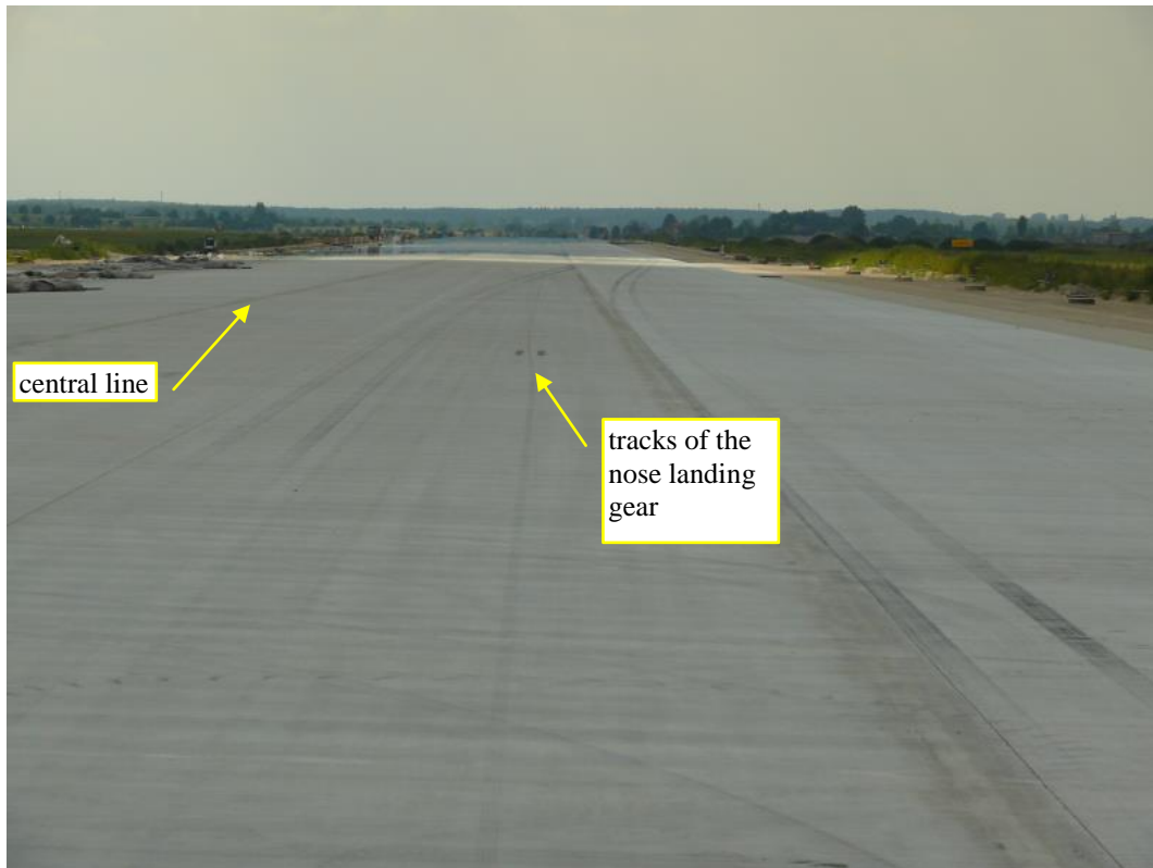
Photo 8. Touchdown tracks of the nose landing gear (~1130 m from the beginning of the runway 27 surface) and a turn at the beginning of the landing roll.
