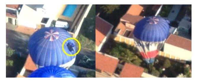
The left photo shows the damage to the upper part of the SP-BPP envelope. The right photo shows SP-BBP landing with the envelope only partially inflated.
