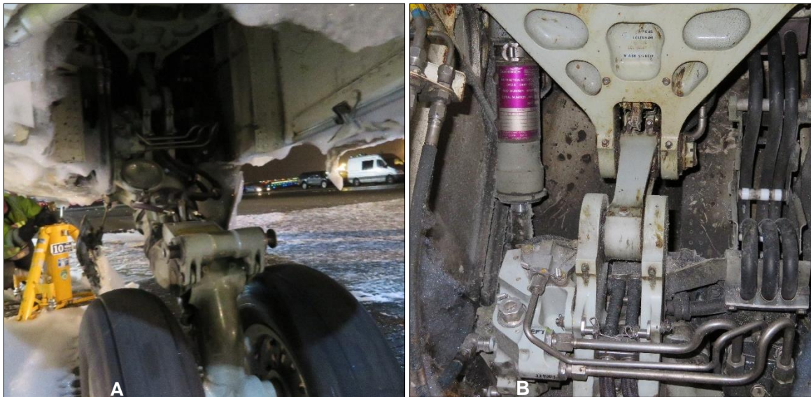
Fig. 26. Lifting the airplane – relative location of the Lower Drag Strut and Upper Drag Strut: A – general view, B – close-up [source: PKBWL].
