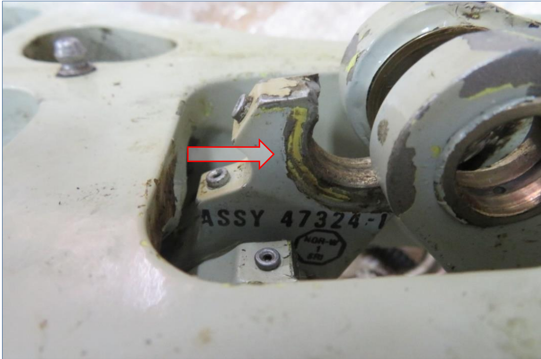
Fig. 36. Lower Lock Link from SP-EQG plane damaged during the occurrence
