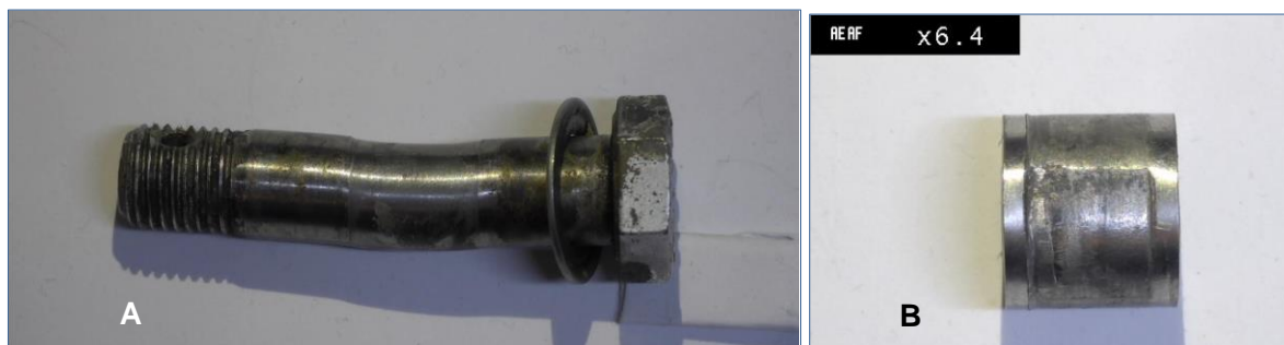
Fig. 32. View: A - bolt (according to DSA CMM 1-1180, PN NAS6206-20D), B - sleeve (according to DSA CMM 1-1160, PN 47326-13)
