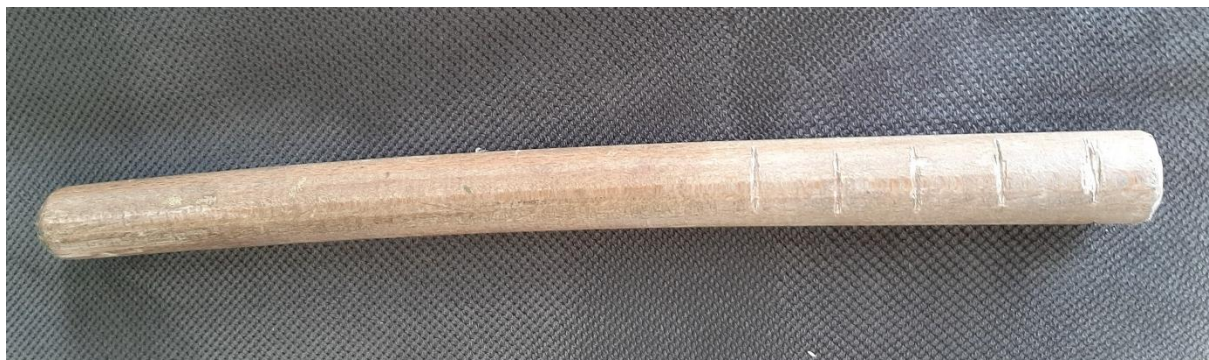
Fig. 14. Wooden pin with cut scale, used to check the amount of fuel in the tank [source: SCAAI]
