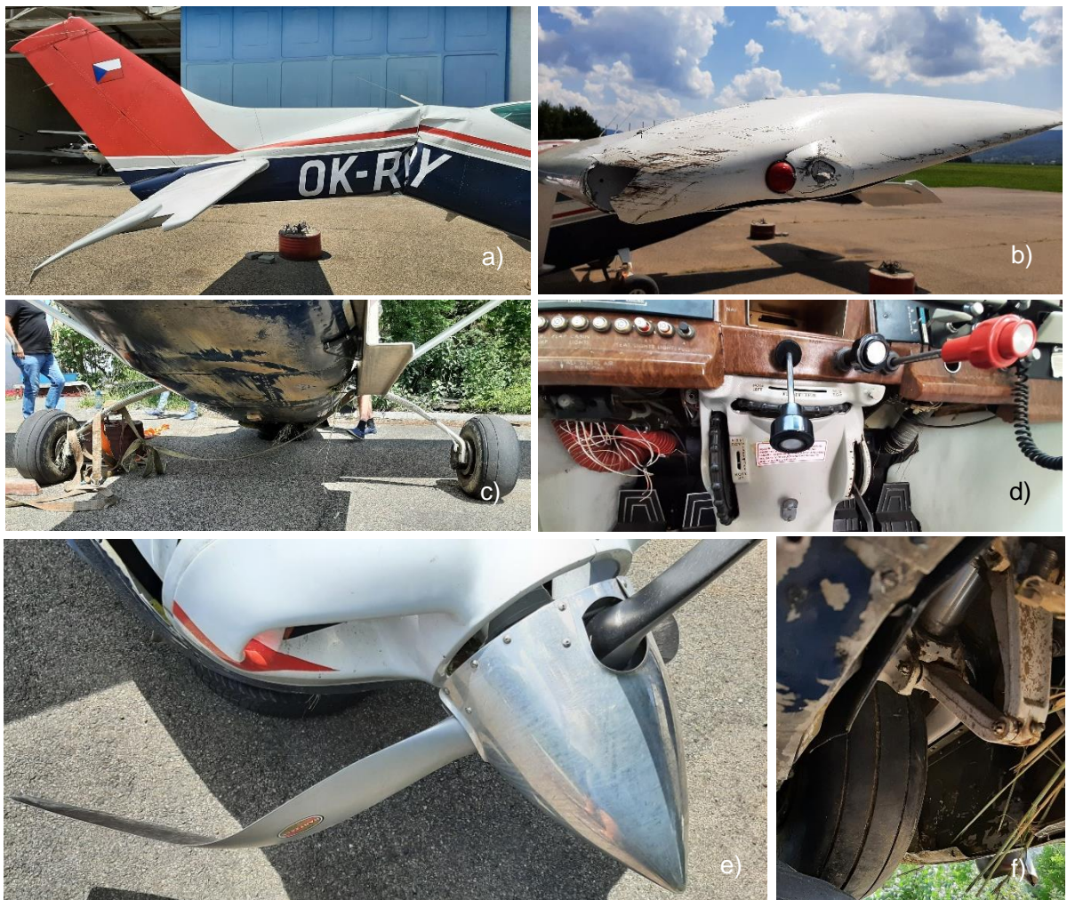
Fig. 3. Damage to the aircraft: a) broken fuselage, b) left wing tip damage, c) scratches on the bottom part of fuselage and main landing gear, d) bend on the throttle lever, e) bent prop blades, f) broken front undercarriage fork, pressed into engine compartment [source: SCAA]
