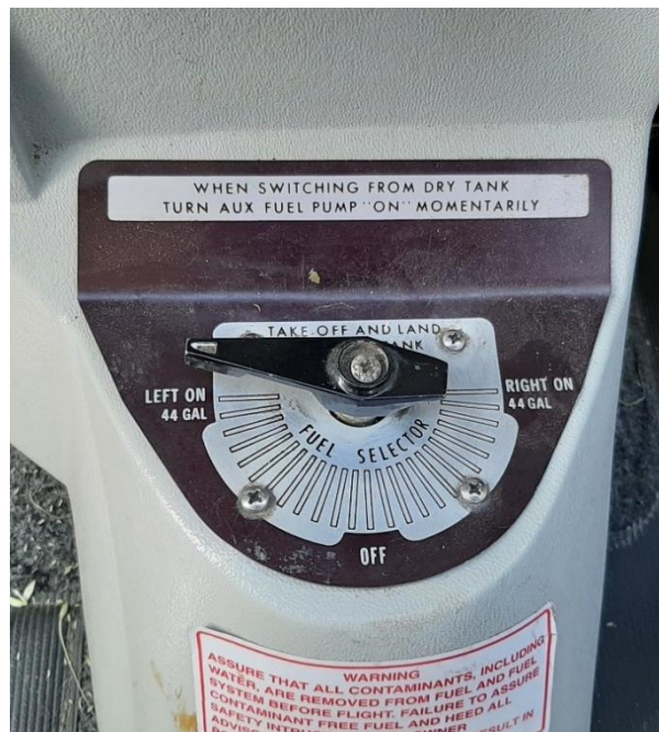
Fig. 9. Fuel valve in the cockpit – the valve knob (in black) controls the fuel supply from the tanks to the engine compartment [source: SCAA]
