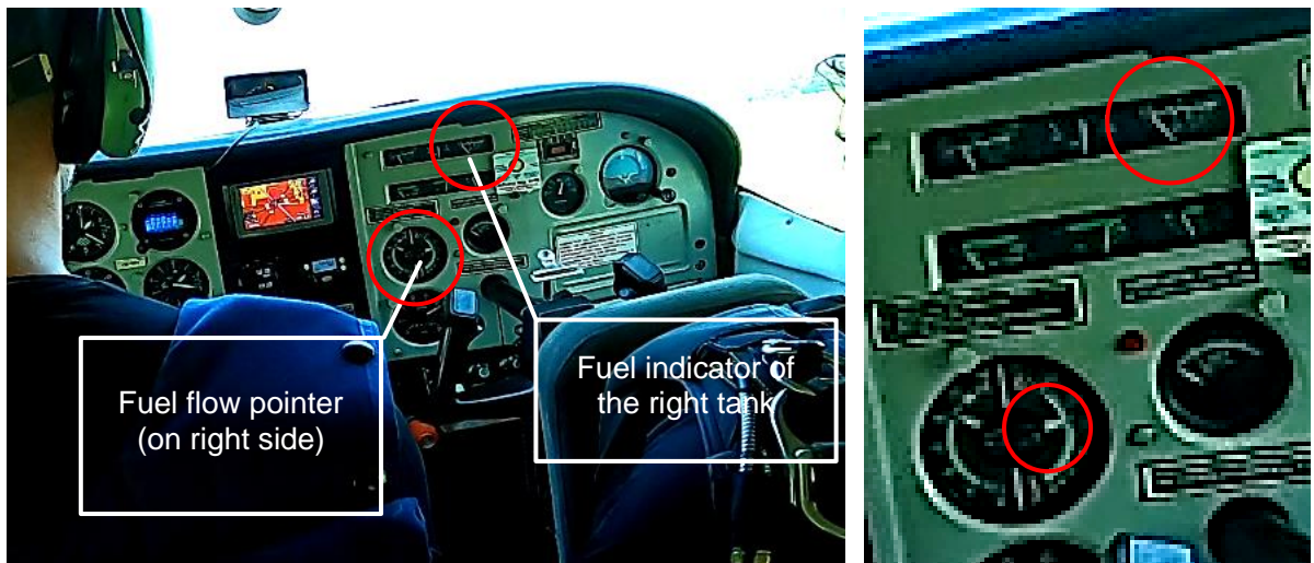
Fig. 12. View of the instrument panel in 7 s from the beginning of run-up. The figure on the right shows the enlargement of a fragment of the instrument panel and marks the fuel meter and flow meter [source: video footage recorded by the camera of one of the jumpers]
