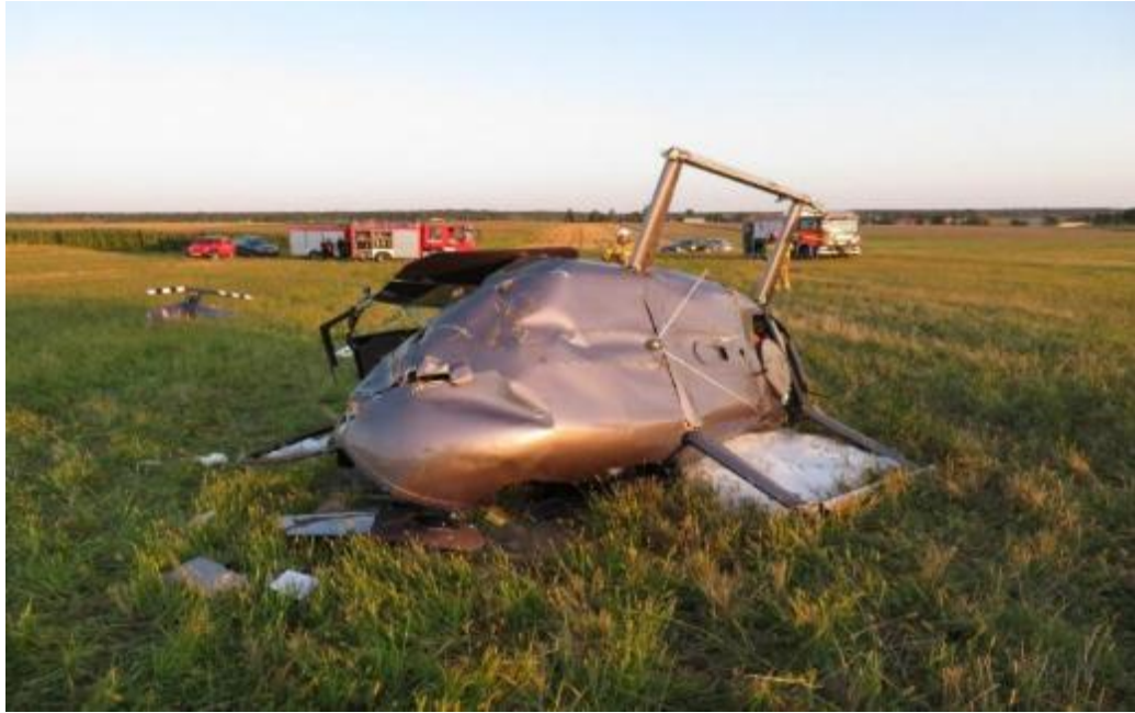
Fig.15. Visible damage to the lower part of the fuselage.
