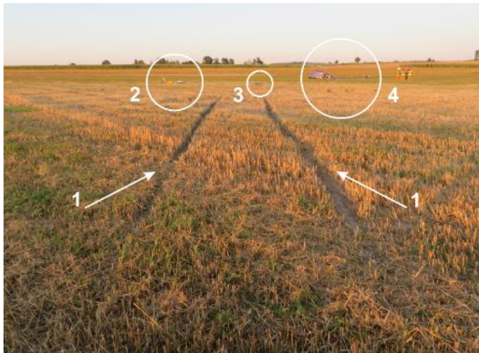
Fig. 11. The crash site as seen from the direction of landing. 1 - traces of touchdown and run-up; 2 - fragments of the lifting rotor blades, 3 – front parts of the skids, 4 – helicopter wreckage with the tail boom and broken tail rotor gearbox and stabilisers.
