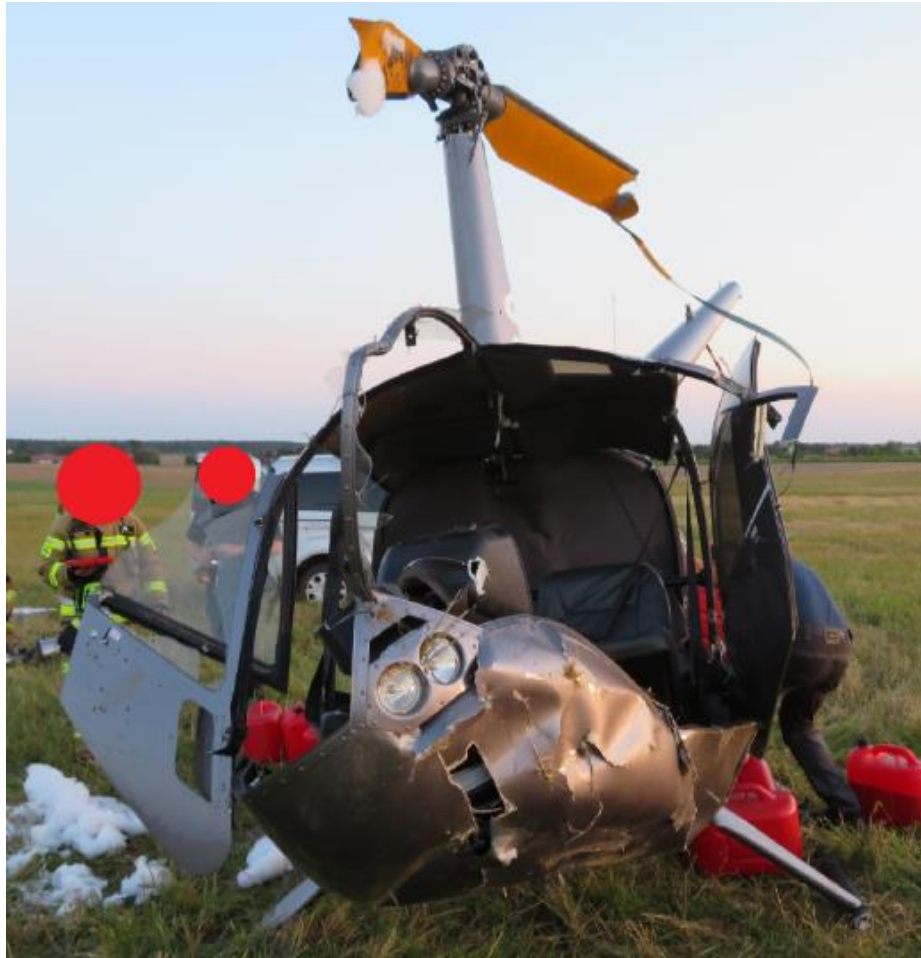
Fig. 13. Deformed helicopter cockpit.
