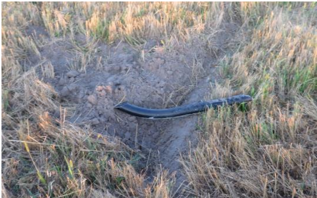
Fig. 16. Separated right skid section.
