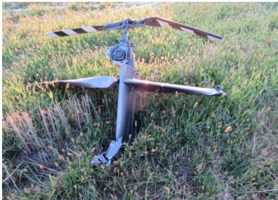
Fig. 14. Separate tail rotor gearbox including tail rotor and stabilisers.
