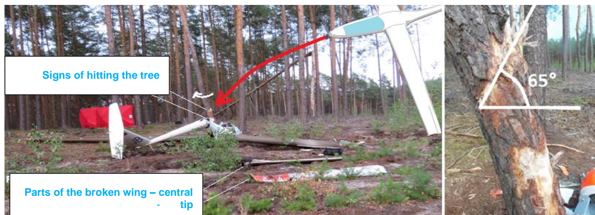
Fig. 7. Probable course of the final stage of the accident. [source: PKBWL].
