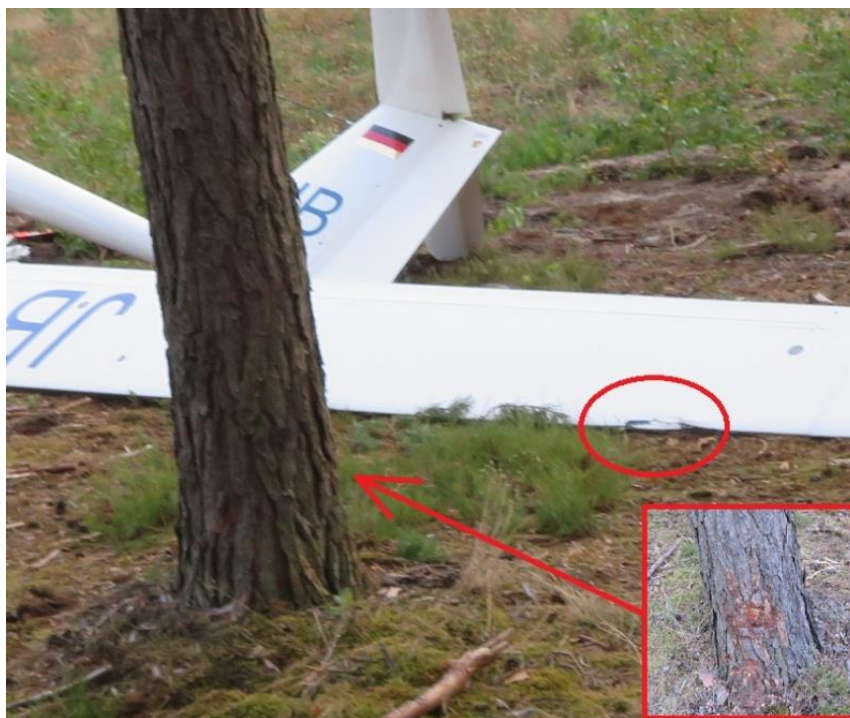
Fig. 8. Indentation of the leading edge of the right wing and traces on the trunk where the wing hit the tree [source: PKBWL].
