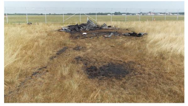
Fig. 11. Accident site. Burnt wreck and burnt grass indicating the direction of the spilling fuel after the impact [source: PKBWL]
